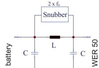
To smooth down the input sine current ( $2xf_0$ ), which is caused by very high input capacity a choke can be connected input sided.
