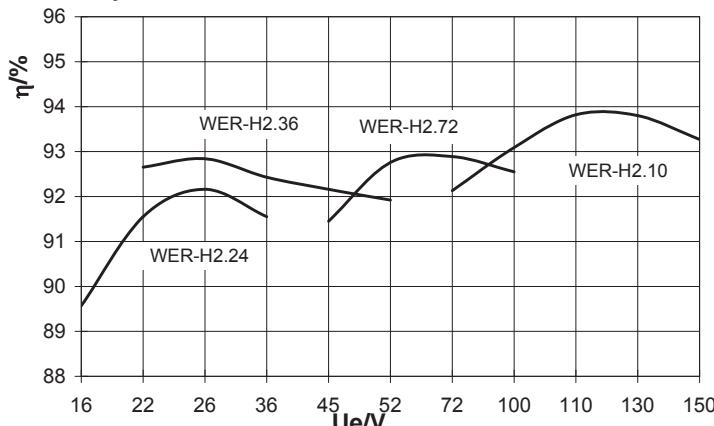
1ph/2ph inverters operate on battery networks in vehicles to supply kitchen equipment, pumps, fans, tools, passenger sockets or similar applications. The new **WER.H2** series generates a synthetic, regulated and short circuit proof 230V sinus output with an output power up to 900VA continuous and 1100VA dynamic.
