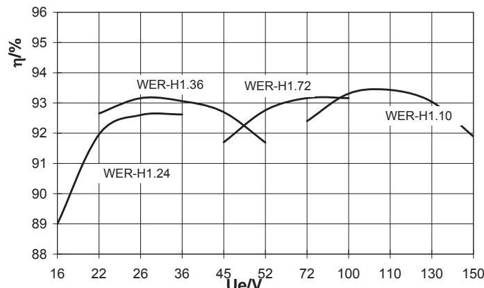
1ph/2ph inverters operate in battery networks in vehicles to supply kitchen equipment, pumps, fans, tools, passenger sockets or similar applications. The new **WER.H1** series generates a synthetic, regulated and short circuit proof 230V sinus output with an output power up to 430VA continuous and 500VA dynamic.
