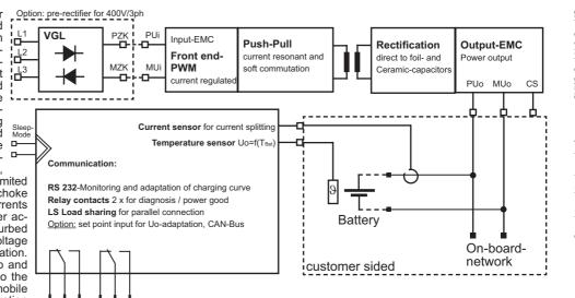
Ventilated operation3), is mandatory and recommended to improve the MTBF. The supply for the ventilation is internally generated by a an integrated auxiliary converter. The input circuit is protected against long term transients (in closed energy systems) without current refection, radio interference suppressed and can deal with chattering over plugging and short-term power failures (auto re-start). Input sided supply voltage ripples of <5% (nominal level) can be processed.
